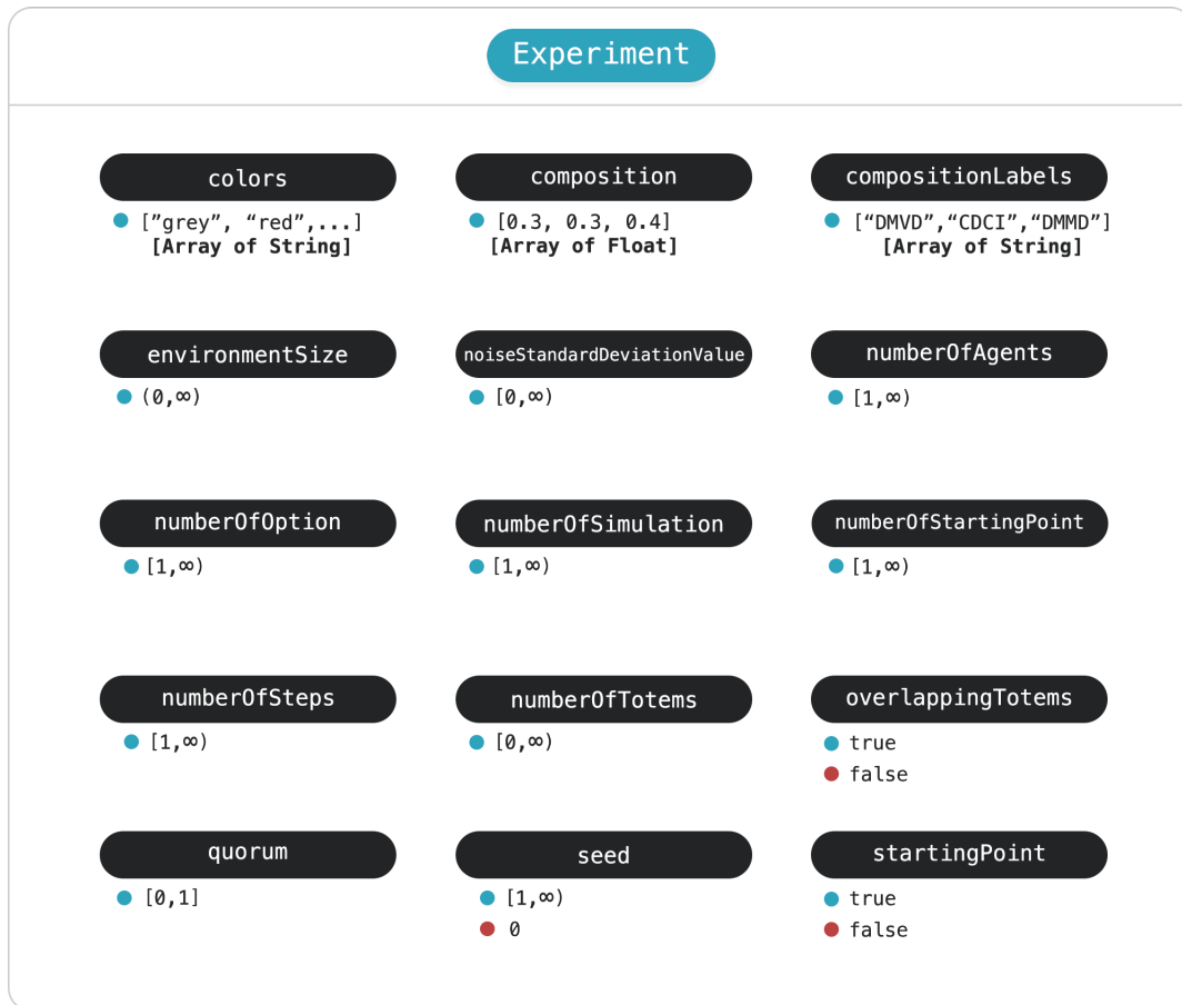
Figure 3.15: Experiment parameters overview, with the black rounded rectangles we indicate the name of the parameters, and next to the blue dots we list the range in which the parameters has to be set or a possible configuration in case of Arrays.
