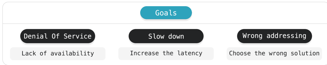
Figure 4.2: Goals of an attack motif, an attack can have three different goals: Denial Of Service (DOS), slow down, and wrong addressing.
